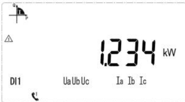
Current total power is 1.234kW
