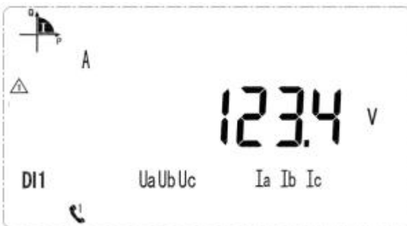
Voltage on A phase is 123.4V
