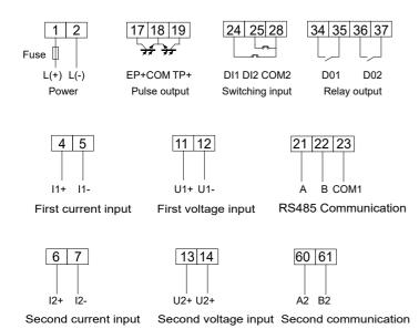
Note: The second DC input channel and DI and DO functions are optional.
