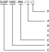
Power Supply: None-AC/DC 85-265V P1-DC 24V,48V Auxiliary function: K-Digital input and outputing /2C-Two way communication(either-or) D-Double DC input channels DIN 35mm rail mounted Registration number DC meter
