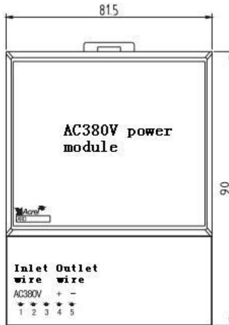
Figure 9 Outline dimensions of AC380 power module
