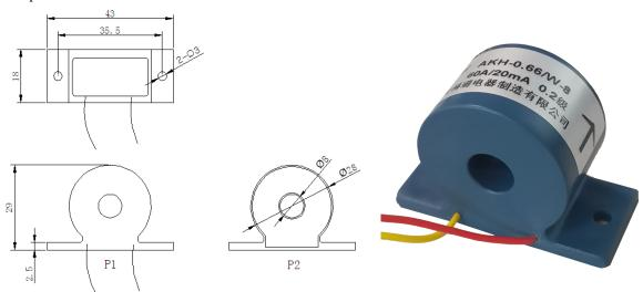
Note: Primary current flow from P1 to P2. The yellow second wiring is S2, the red is S1. The outlet length is  $2m \pm 10$ cm.
