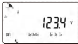
Voltage on A phase
