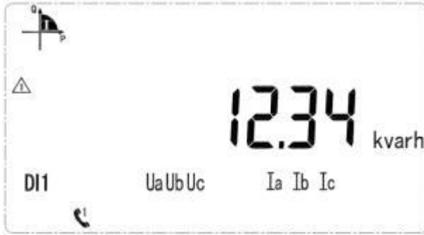
Current forward reactive energy 12.34kWh
