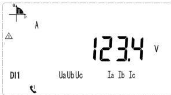
Voltage on A phase is 123.4V
