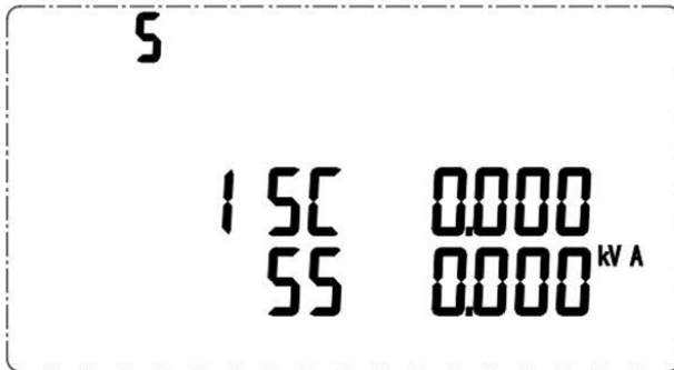
Apparent power S_c and total apparent power
